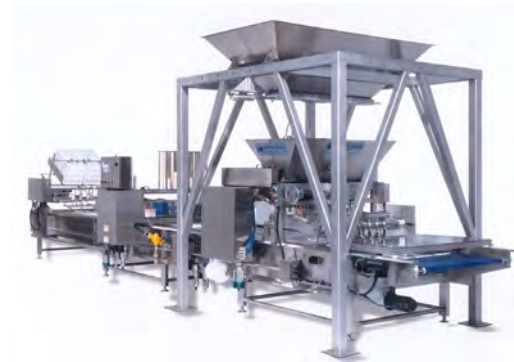
Fully automated high volume pre-bake muffin line
