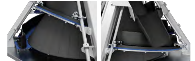
Special designed infeed track, manually adjustable
